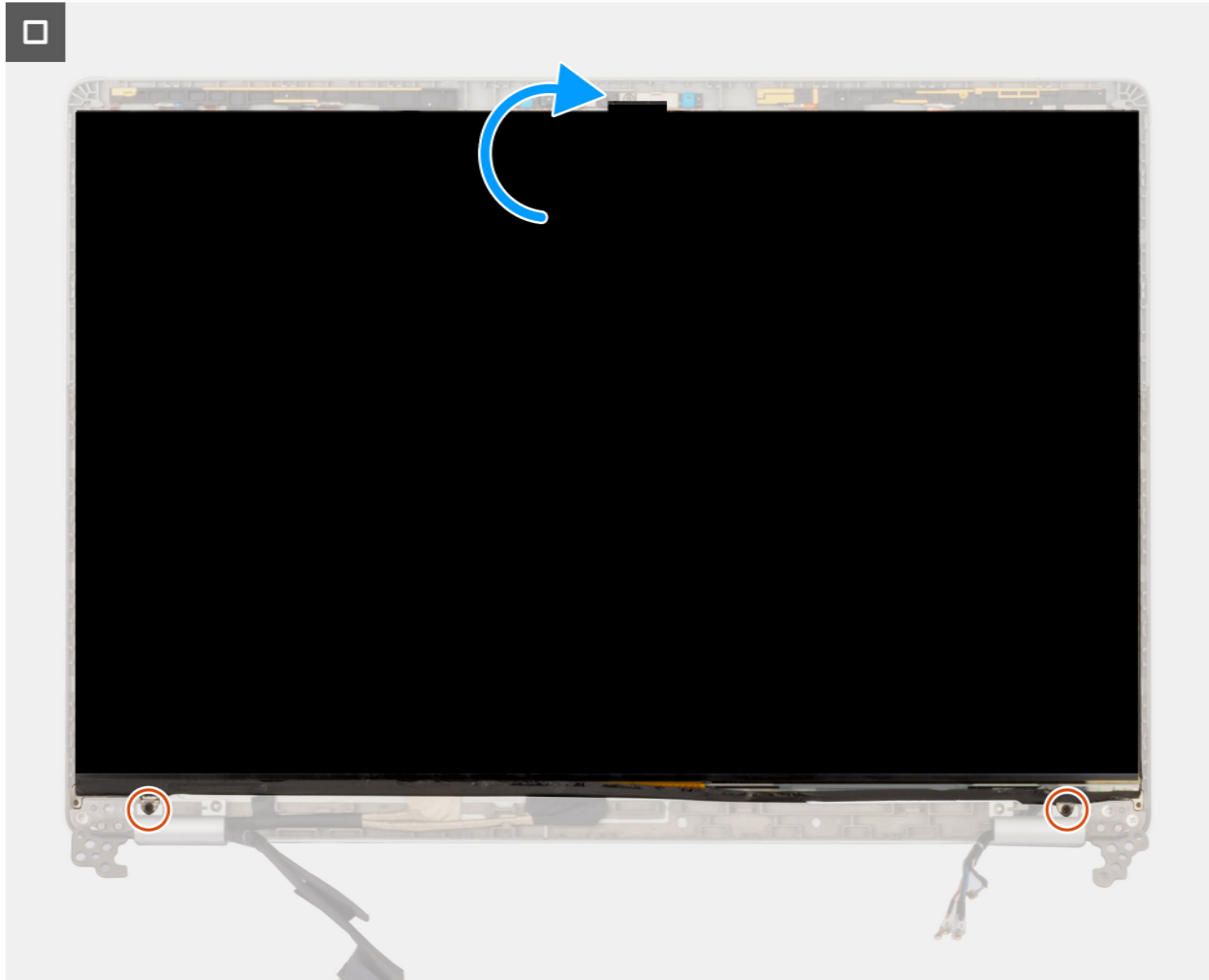
Figure 33. Installing the display panel
