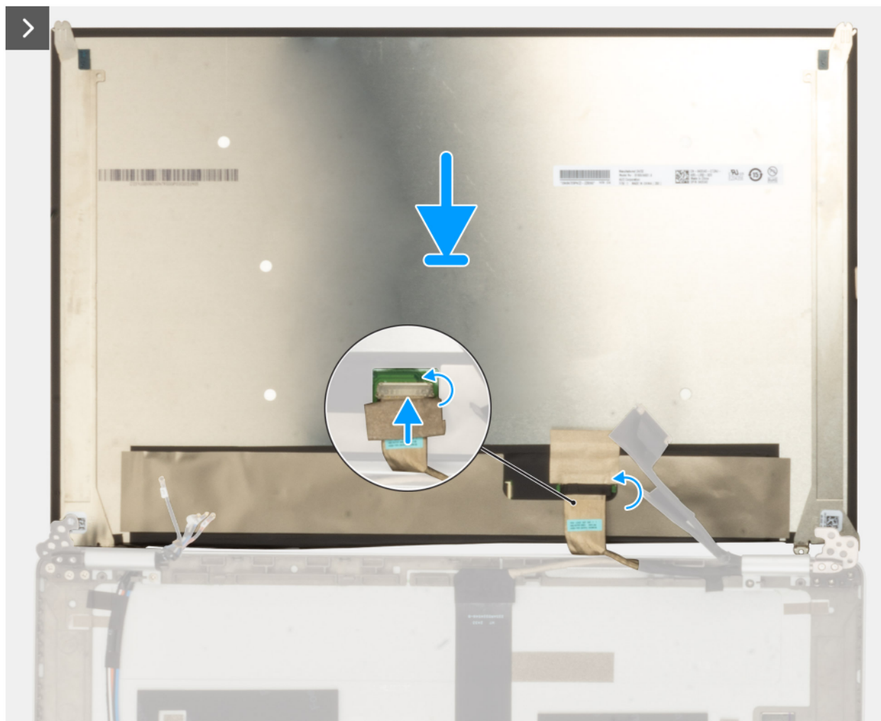
Figure 32. Installing the display panel
