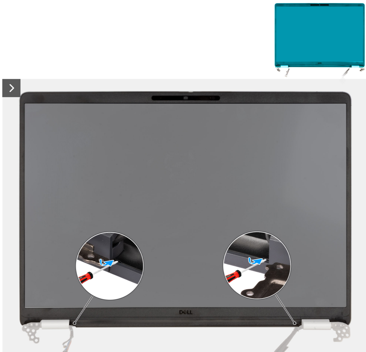
Figure 24. Prying the plastic bezel
