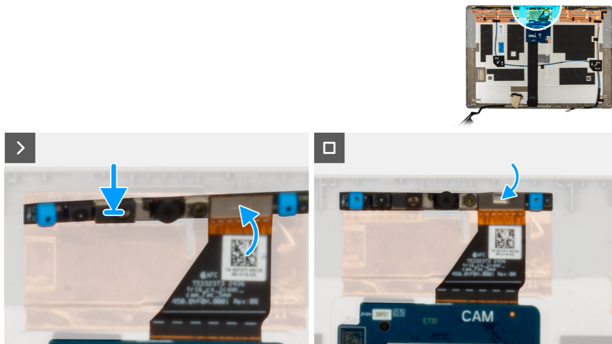
Figure 39. Installing the camera module display cable
