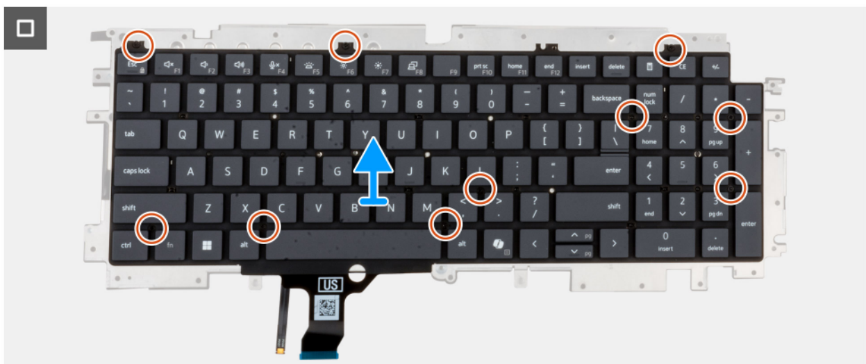
Figure 59. Removing the keyboard
