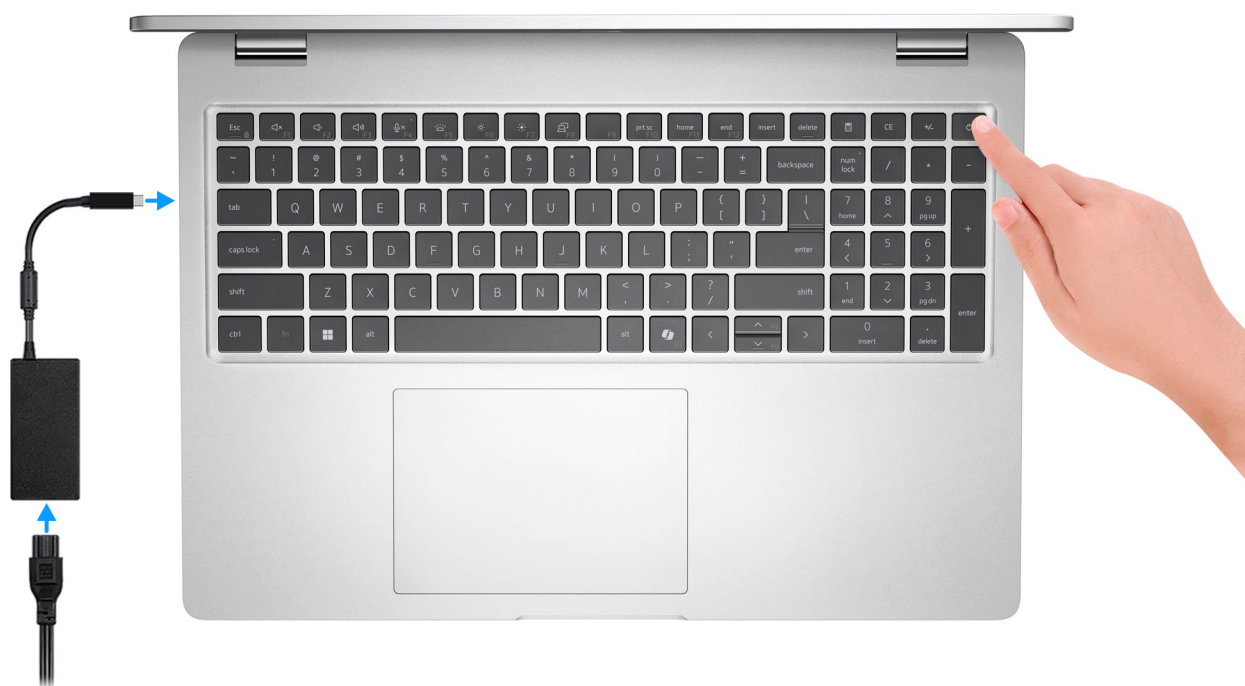
Figure 1. Connect the power adapter and press the power button.
